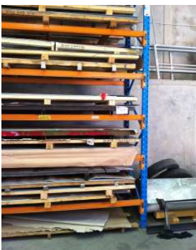
1. Racking for sheet storage
