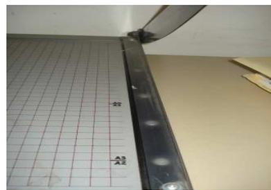
Figure 2 Guillotine with guard in place
